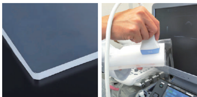
High transparent and ultra-soft plate-like phantom. It is possible to train different fat layers by changing the thickness.
