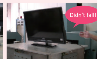
M9 seismic wave reproduction test conducted.
