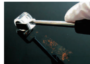
Transfer the dusts which removed by adhesive roller to Semiconductive gel sheet.
