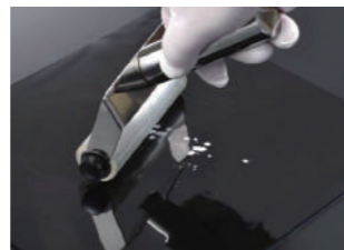
Transfer the dusts which removed by adhesive roller to Semiconductive gel sheet.
