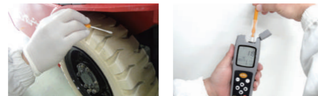
Measure the remained dirt of forklifts that had run for a minute indoors. Then the same forklifts ran on the mats and measured a dirt again.
